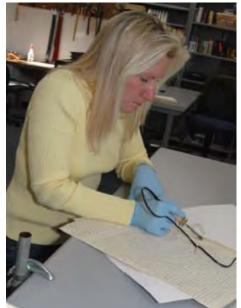
A Hot Tools tape remover softens adhesive to allow for removal. Dial-Temp controls the transfer of heat and guards against scorching.
